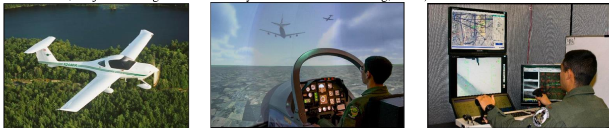
FIGURE 4. URT aircraft and flight simulators. Left , the Diamond DA-20 is used during RFS; center , the T-6 flight simulator is used during RIQ; right , the PRIME is used during RFC (Adapted from briefing, Lt Col Jack Stallworth, Headquarters Air Education Training Command [AETC], 558 th Flying Training Squadron Commander, subject: Undergraduate Remotely Piloted Aircraft Training, 2016.)
